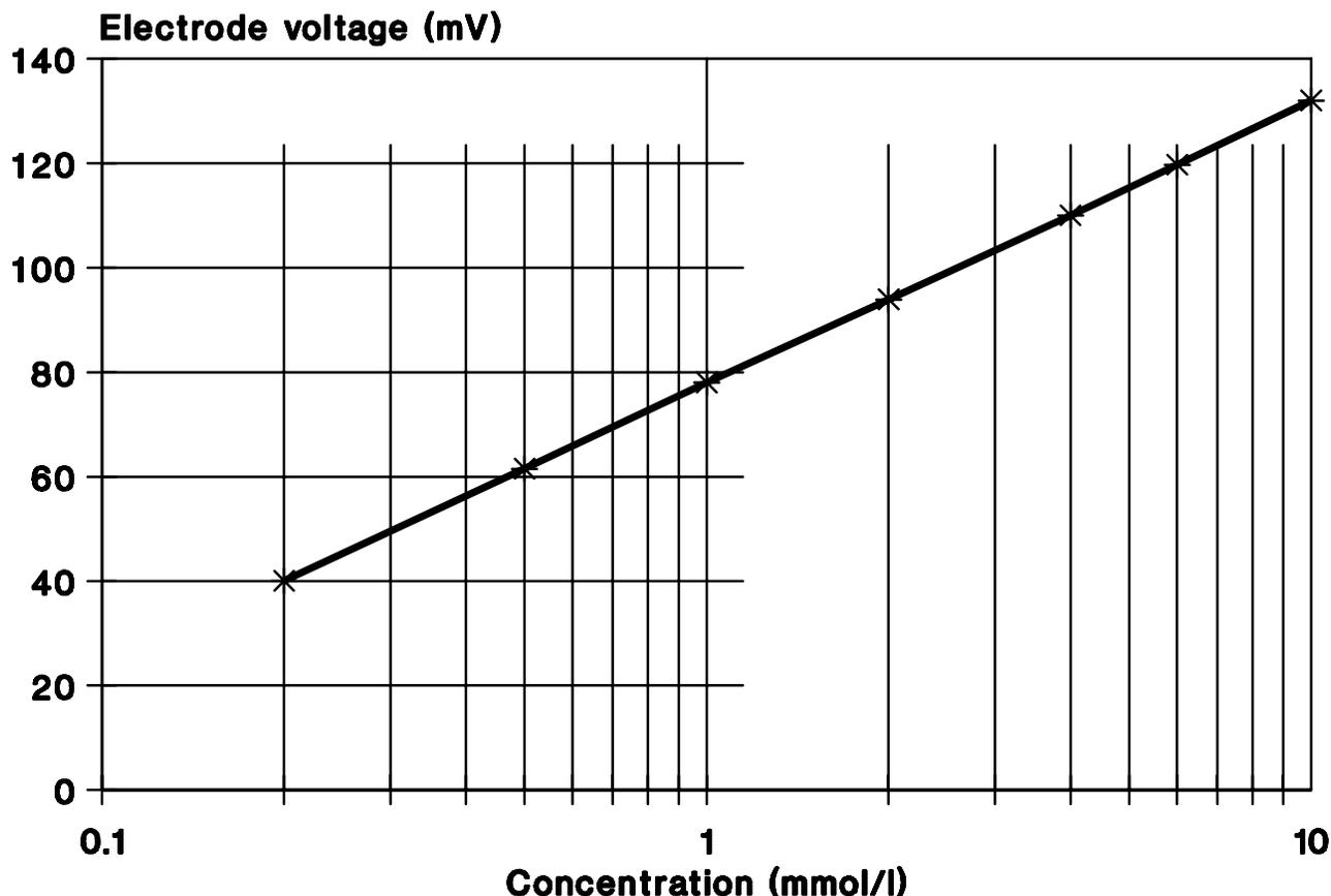
Fig. 3 Concentration - mV relation of a  $K^+$  electrode model 601
