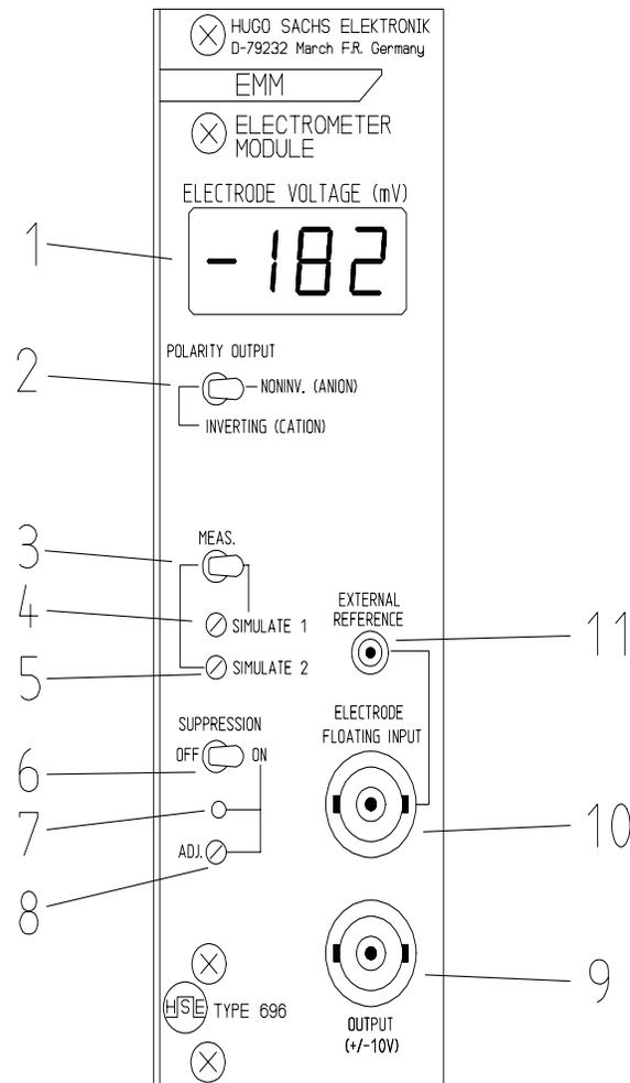
Fig.3 Controls on the front panel
