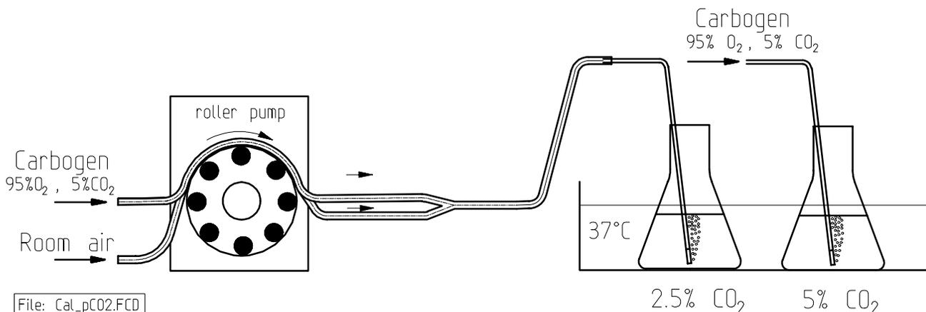
**Fig. 3:** Calibration setup for pCO<sub>2</sub> electrodes
