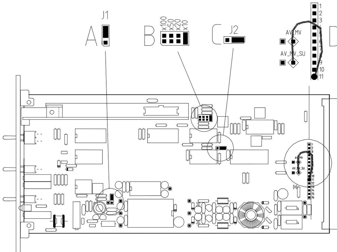
Fig. 2: Position of the internal links
