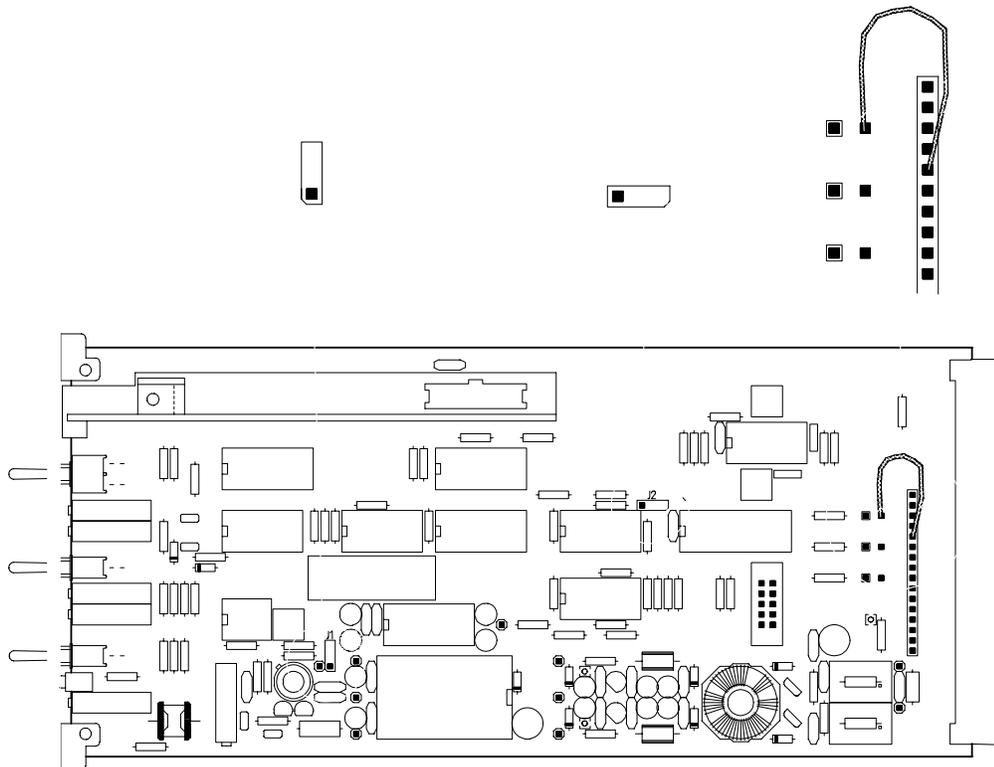
Fig. 2: Position of the internal links
