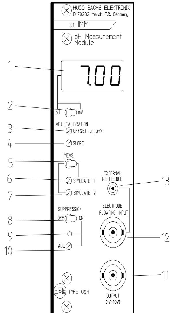
Fig.3 Controls on the front panel
