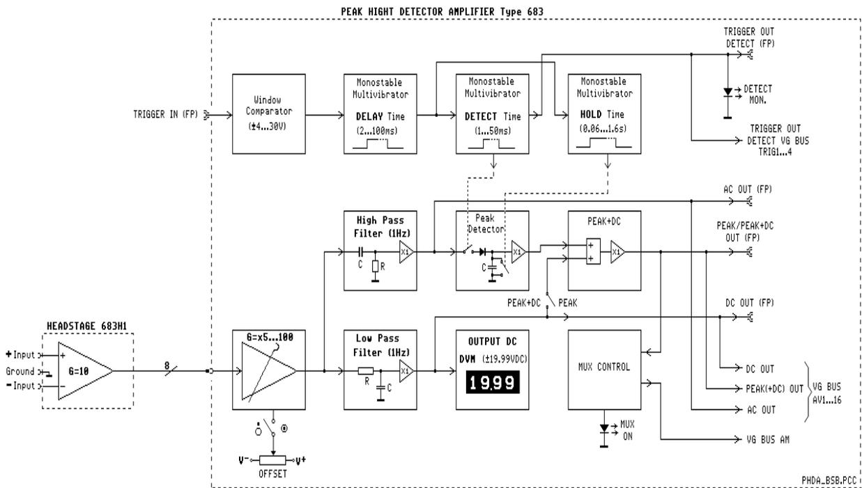
Fig. 5: Block diagram of the Peak Height Detector Amplifier PHDA
