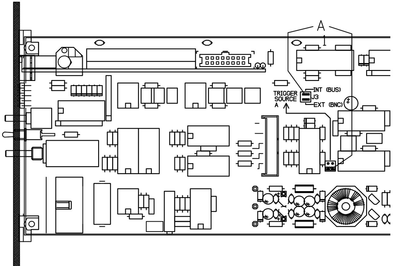
**Fig. 8:** View of circuit board of the PHDA. Before installing the module in the housing the links A...D have to be determined. Note details in the text!
