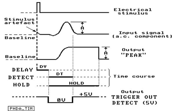
**Fig. 4:** Time course during capture of the peak amplitudes. Note: negative signals are not recorded.
