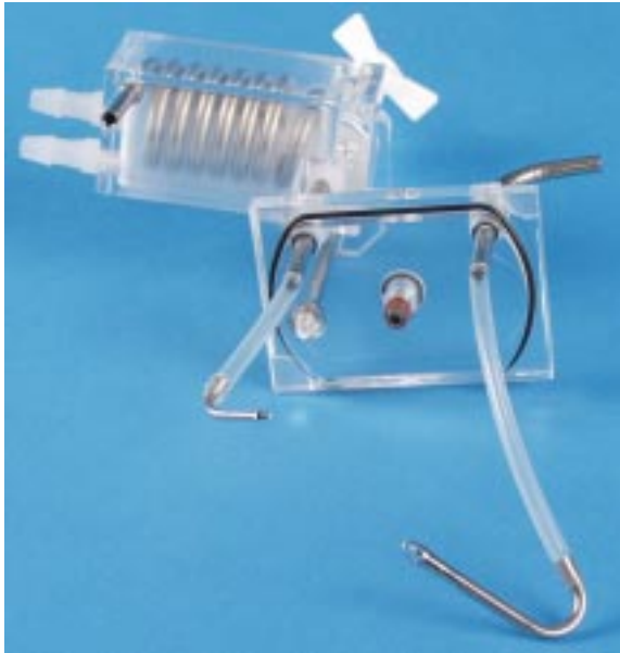
Standard Lid as removed from the IPL2
