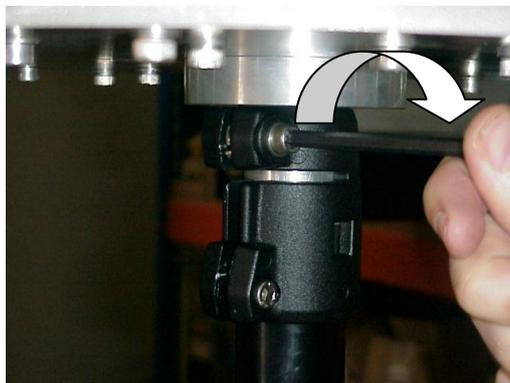
Figure 7. Securing the platform to the support.
